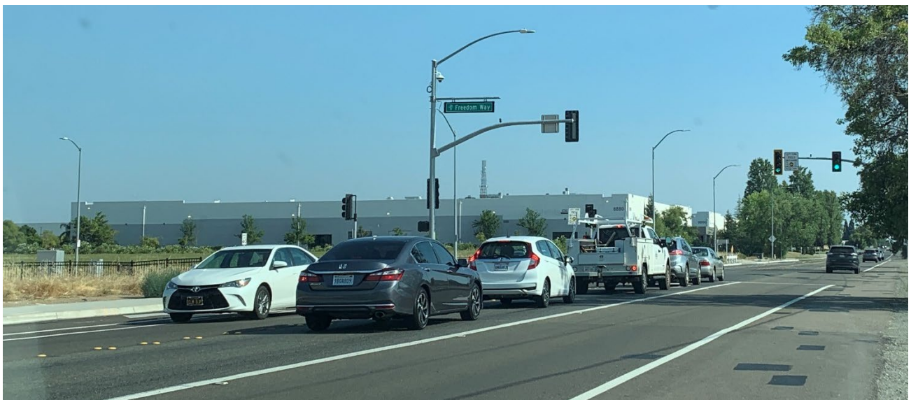
Image 3: Maximum queue of 5 vehicles in southbound left-turn lane during PM peak hour on Monday, July 11, 2022 (note that the protected green arrow had been activated)
